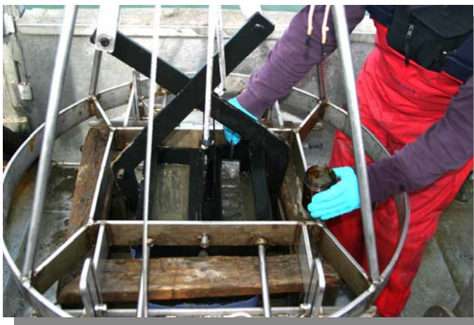
Van Veen grab with sediment sample
